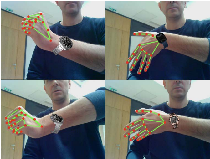
Fig. 11. Visualization of extreme hand poses and unusual orientations, relative to the forearm, demonstrating the limitation where the watch appears to “float” or distort in relation to the wrist.
