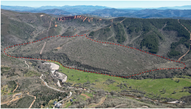
Fig. 8 The scale of the mining works. Mining site of La Leitosa (León), exploited using the arrugia ( ruina montium ) method, with an associated fan of tailings resulting from the washing and recovery of the precious metal.
