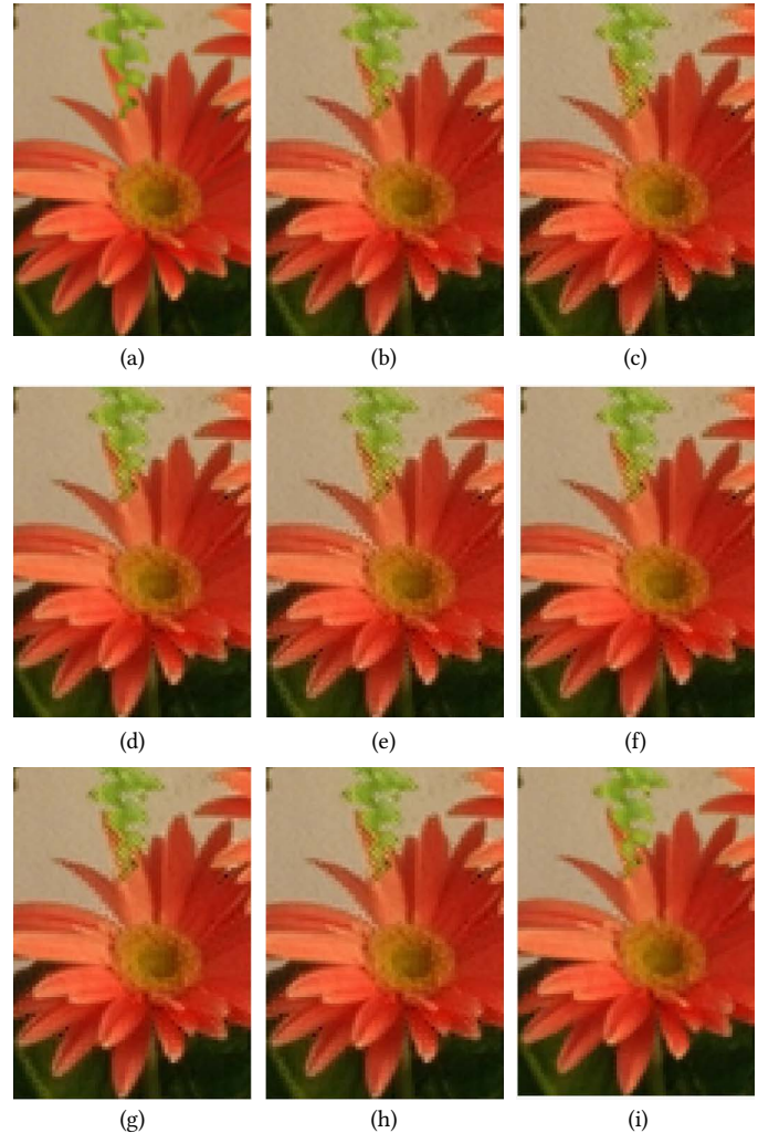
Fig. 7. (a) Part of the original McM #6 image. Perceived image quality comparison using various deinterlacing methods: (b) AFD, (c) VCD, (d) HOI, (e) ESF, (f) EDAEP, (g) ECI, (h) GD, and (i) proposed method.
