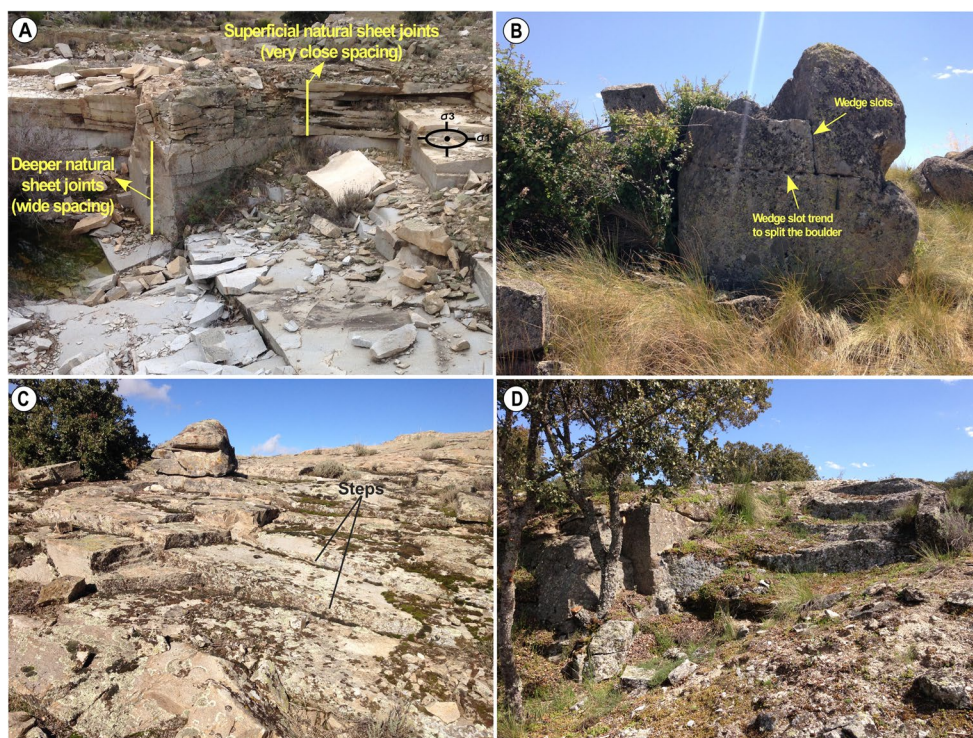
Fig. 8 (A) Distribution of sheet joints in the FBG, with very close spacing in the first few meters and wider spacing at depth. Two of the main axes (sigma 1 and sigma 3) of the stress ellipsoid are shown, corresponding to a non-hydrostatic stress resulting from load release due to erosion, which in this case breaks the rock into more or less subhorizontal planes. (B) Surface mining of a PCBG granite block using traditional methods. C and D) Fronts of historical quarries quarried on a slope using traditional methods, in FBG (C) and PCBG (D)
