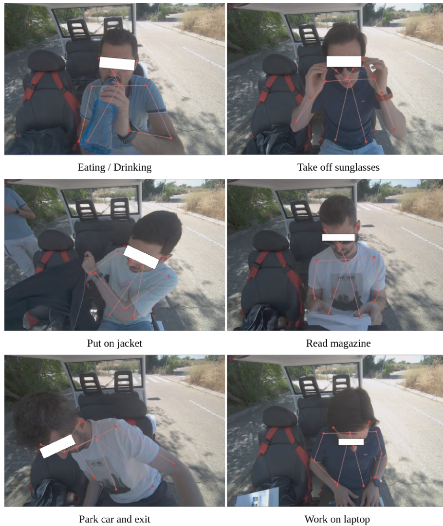
Figure 6.7: Example frame for the 2d representation in the image plane of the pose obtained by the ZEDX mini for six different actions.
