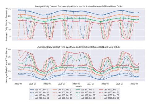
**Figure 12.** Time plots for daily contact frequency (**top**) and daily contact duration (**bottom**) for the 16 Mars orbits.
