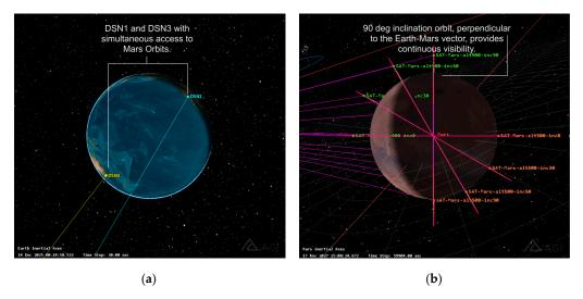
**Figure 13.** Scenario snapshots with two simultaneous DSNs in sight in (**a**) and 90-degree inclination orbit with permanent sight in (**b**).
