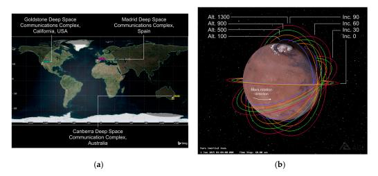
**Figure 5.** DSN and Mars orbit scenarios. (a) NASA's Deep Space Network (DSN). (b) Mars orbital scenario and parameters.
