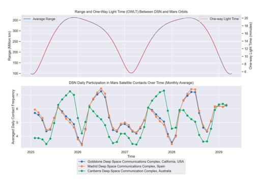
**Figure 10.** Range, OWLT (**top**), and participation of NASA's DSN ground sites (**bottom**) in the contacts between Earth and Mars segments.
