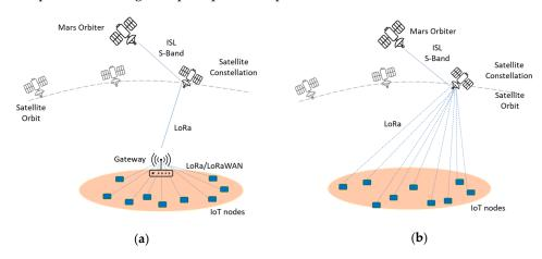
Figure 3. Communication models for nodes: (a) ItS-IoT and (b) DtS-IoT [14].
