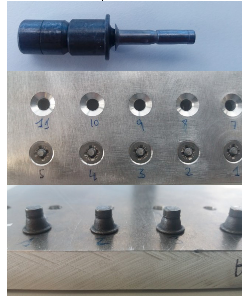
Figure 1 MONOGRAM CL-II blind fastener (top), probe front (middle) and back (bottom) with fasteners installed
